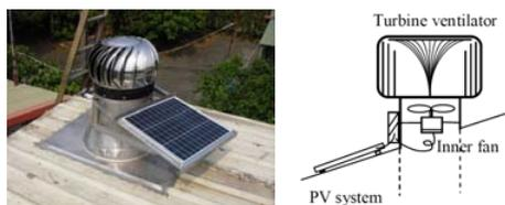
Fig. 1. The Hybrid Ventilator developed and investigated in this study.
