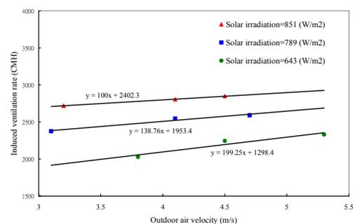
Fig. 3. Ventilation rate variations of Hybrid Ventilators under different outdoor wind velocities (in the same sunlight exposure).
