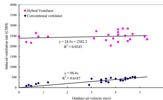
Fig. 2. Ventilation rate variations between a conventional ventilator and a Hybrid Ventilator affected by outdoor wind velocity [4].
