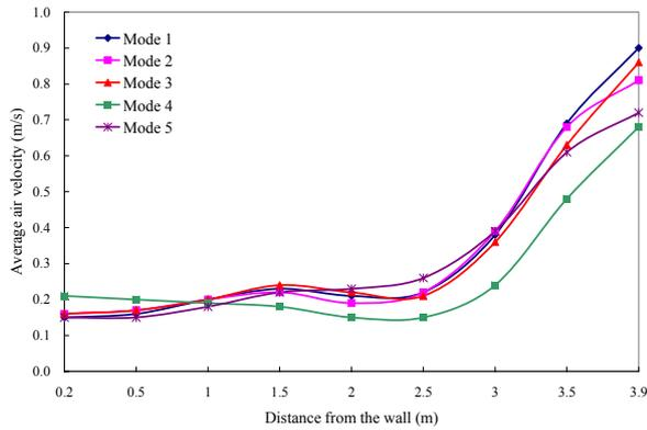
Fig. 6. Average indoor air velocity of the 5 Modes between  $Y=0.2$  m and  $Y=3.9$  m.
