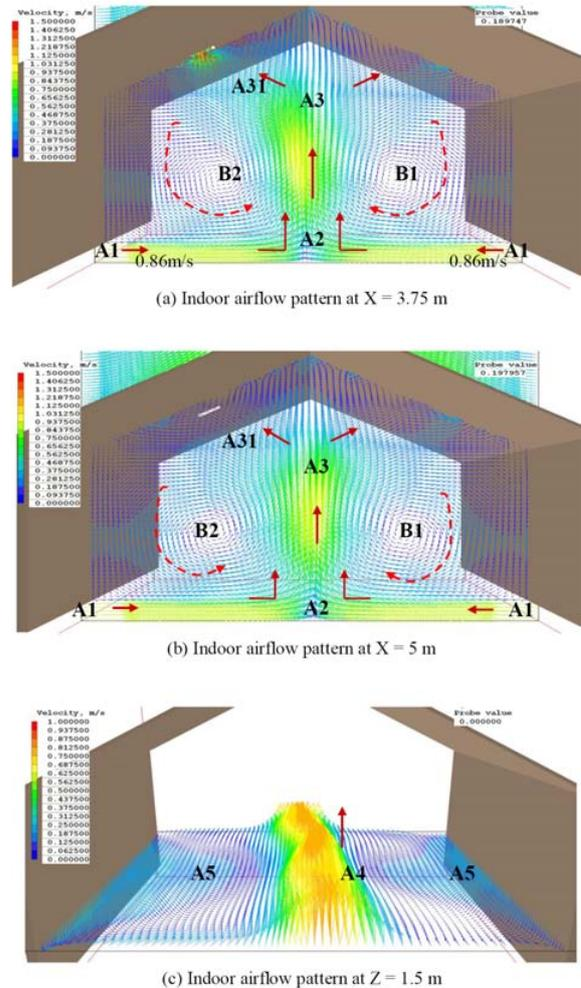
Fig 5. Flow patterns of the interior of Mode 5 at  $X = 3.75$  m,  $X = 5$  m and  $Z = 1.5$  m, respectively.
